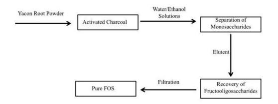
Fig. 1: Schematic process for the separation of fructooligosaccharides from yacon root
