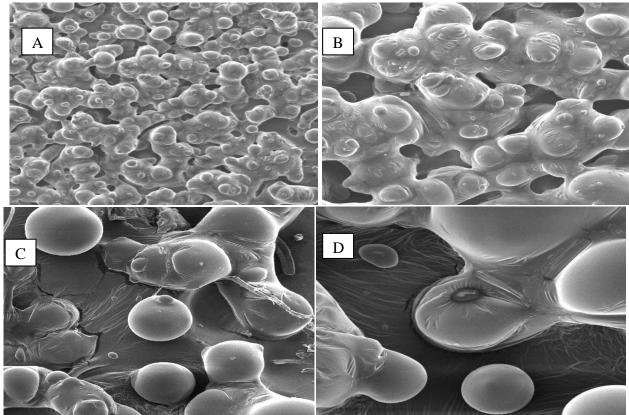
Fig. 2: SEM image for Fructooligosaccharides from yacon root powder, image A and B are commercial FOS with magnification of ×250 and ×500. Image C was yacon FOS under magnification ×500. Image D was yacon FOS with magnification ×1000 to view as single compound for observation after freeze-dried.
